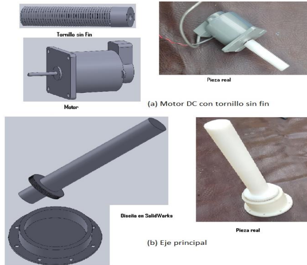
Fig. 6. (a) DC motor with endless screw, equivalent to n_1=1 , (b) Principal axis equals n_2 = 86 . The DC motor uses an incremental encoder, resolution 400 pulses.
