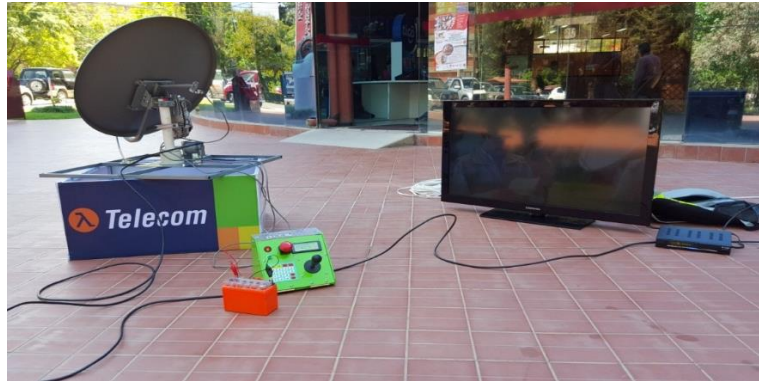
Fig. 10. Final prototype, performing tests with a DVB-S2 receiver with a frequency of 11670 MHZ, symbol rate of 150000 Ksps and vertical polarization.
